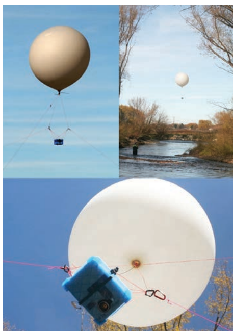
Figure 3. The TIR balloon platform comprises three main parts: the balloon, camera case, and tether system.
